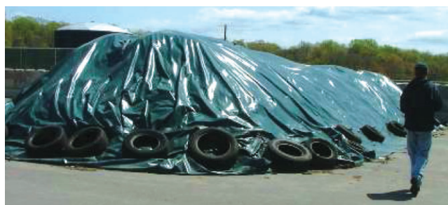
Figure A-3: Fabric-covered ASP system in Howard County, MD. This is a negatively aerated AC Compost System from Engineered Compost Systems (ECS). Feedstocks are yard trimmings and food scraps collected from residential sources. The initial capacity is 7,500 tons per year, but an expansion to 45,000 tons per year is planned.
