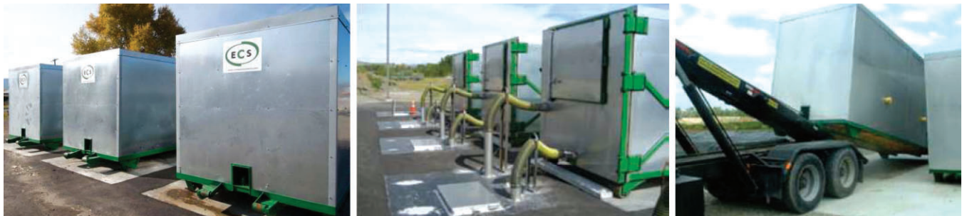
Figure A-9: ECS containerized CV Composter uses insulated 40 cubic yard vessels with stainless steel interiors Photo credit: Engineered Compost Systems
