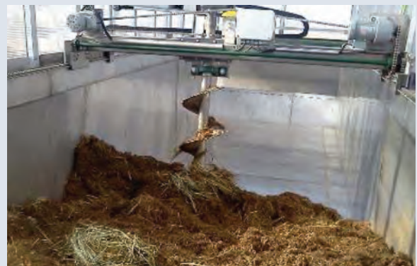
Figure B-2: Auger inside GMT Earth Flow
