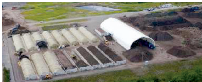
Figure A-4: GORE Micropore fabric-covered ASP
