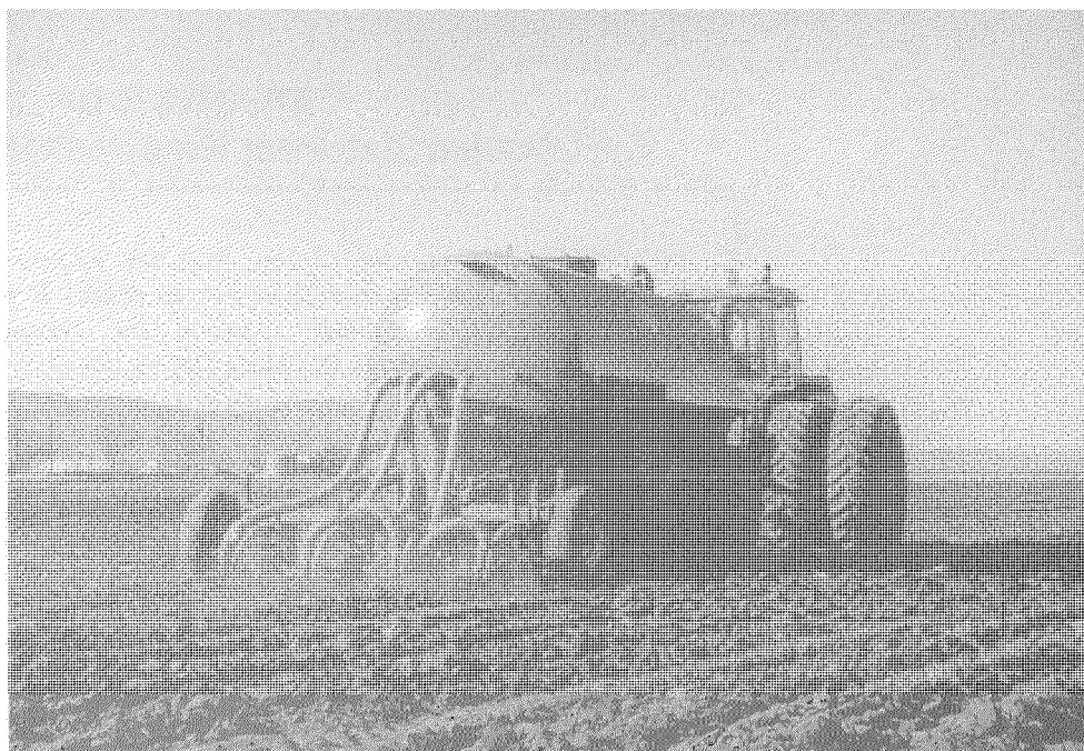
Anaerobically digested biosolids from Los Angeles are injected into the soil in California.
